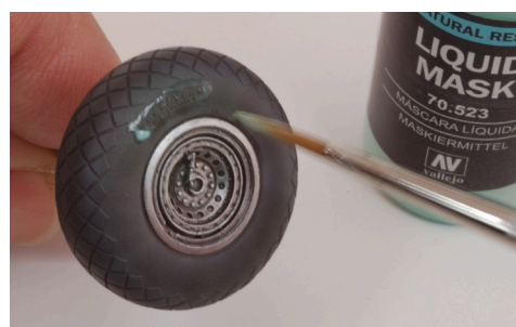
12 In case the tire has the logo of the manufacturer, or imprints of numbers, etc., we proceed to outline these with Liquid Mask 70.523.
