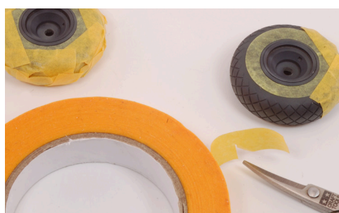
7 The whole tire is covered with masking tape.
