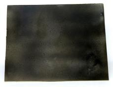
1 The Surface is primed with 3 thin layers of Surface Primer 73.602. NOTE: there is no need for the layers to be homogeneous, as this will provide greater realism when colors are applied to simulate wood.
