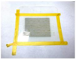
With ST-TX 006 Wood Texture N°1 and masking tape, the stencil is fixed to the surface.
