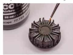
The central block of gears is brush painted with Metal Color 77.723 Exhaust Manifold.
