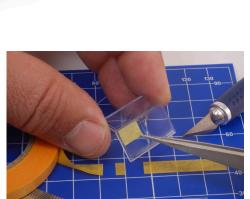
A piece of masking tape is cut slightly shorter than the size needed; for example: if 8mm are needed we subtract 1mm.
