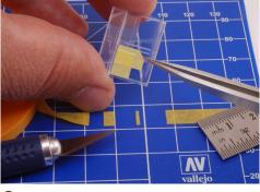
Again, a piece of masking tape is cut slightly shorter than the size needed. A cutting mat and a new blade in the cutter are essential to obtain a precise result.
