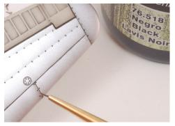
The panel-lines and studs are profiled with Model Wash Black, 76.518.
