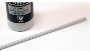
A metal tube is cut into the desired length. The tube is primed in Surface Primer 73.601 Grey Primer.
