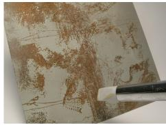
The surface is moistened slightly to allow for easy removal of some of the paint and show the oxide underneath.
