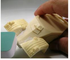
When the surface is dry, it can be sanded using a fine grit sandpaper, in this case 600/1000. This results in a clean and smooth finish.
