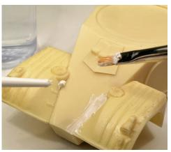
A small amount of Plastic Putty is applied, and it is smoothed out on the surface with a brush moistened with water.
