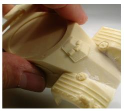
**6** To detect possible defects in the sanding, apply a coat of primer which will reveal any irregularities.
